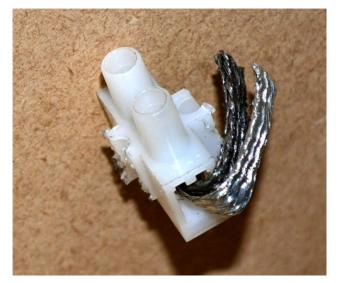
Chocolate block connectors used for a "Power Tap" under the track, quick, simple, clean and no solder joints which may increase resistance over time.
