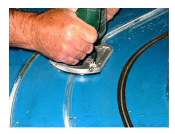
Trim using a wing cutter the full width of the braid bed with a suitable pilot guide pin (in this case 3mm) to machine the braid bed totally flat and to the same height as the unaffected areas. The affected areas trim very easily with no snatching or chipping (use a sharp HSS or carbide cutter.)
