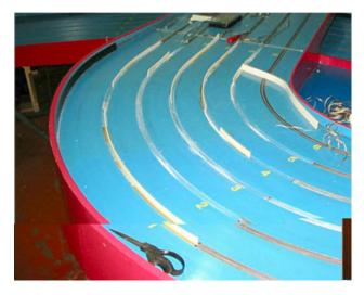
Lift Braid, clean crud from slot and braid bed, vacuum clean and insert Silicon strip into Full depth of the slot. Apply mixed Epoxy to Affected areas with a syringe. Epoxy fills any Irregularity in slots and braid beds. Repeat if necessary where epoxy is absorbed by the MDF. Ensure the Silicon strip is a couple of inches Longer than the area to be treated to ensure Epoxy does not fill the slot by bleeding past the Silicon strip.
