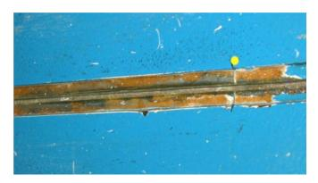
Once epoxy has cured (24 - 48 hours), lift out The Silicon strip (this will not stick to the epoxy). See how the epoxy has formed precisely to the Silicon strip giving a perfect 3mm wide slot with smooth edges. The epoxy Self levels, with a slightly raised edge against The Silicon Strip.
