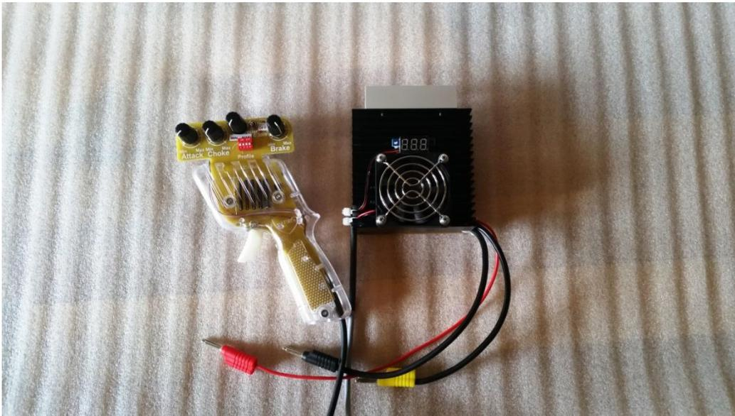
25 steps, all equal size. Trigger response can be adjusted using profile switches to make controller softer or more aggressive.
