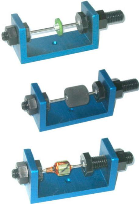
With increased roll height it is possible to balance tyres up to 28mm diameter, gears and even static balance home wound armatures with shaft lengths between 21& 50mm by just grinding a fine point on the shaft ends.
