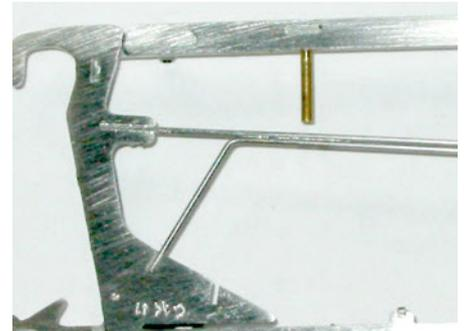
Twin 0.032" rails. This removes the "rear steer" from the chassis and stiffens the flex. Both rails fit perfectly into the rear receptors which are designed to take 1/16" diameter tube. Rails at the front solder into the existing front receptor and the front "lead wire loop" slot.
