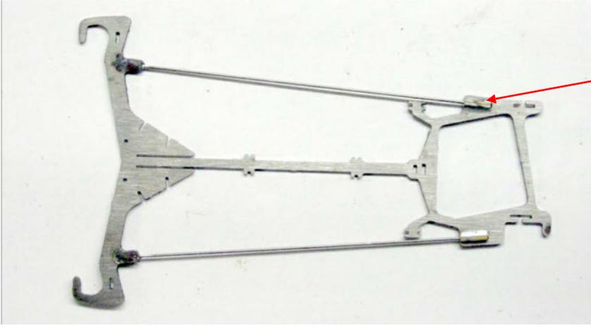
Start with the centre section - cut two short pieces of K&K /16" o.d. Brass tube and solder into the rear rail mounts.
