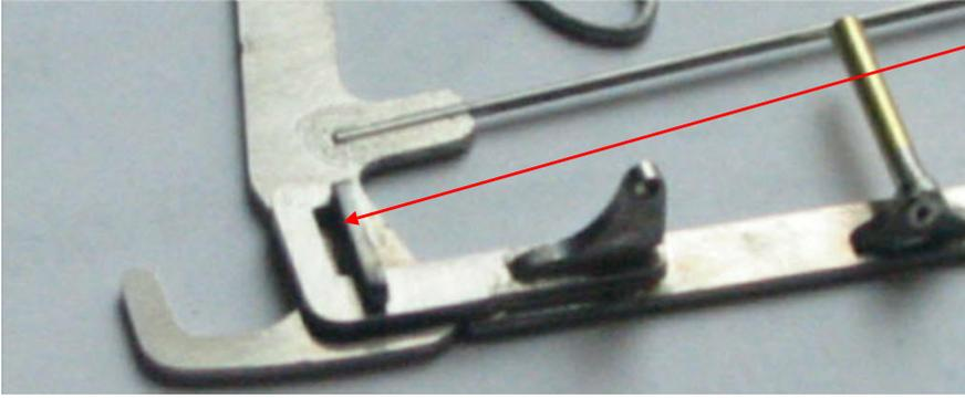
Solder the front upstop into it's slot in the front T bar. Ensure yo remove any excess solder around the upstop so the pan upstop plates do not fowl on the upstop. Locate the The upstop plate and Front wheel mount/ upstop plate key in the front slot in the side pan. Solder in place. Ensure that pan moves freely without fowling. Solder the Anti deck plates into the rear of the pans.
