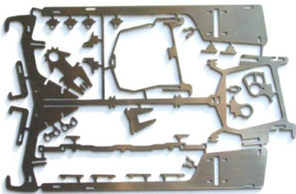
When trimming components ensure to only trim joining sprags and not the components themselves
