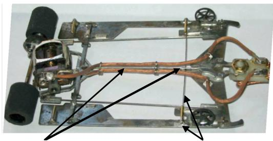
New versions of this chassis now feature a 0.047 centre rail, solder this at the back and also to the two lead wire retainers and the rear of the guide plate. It is also advised to use stainless steel pin tube in the pin mounts.
